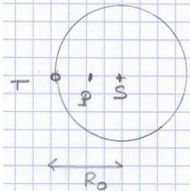
1) PFD  $-\frac{M_0 v_0^2}{R_0} = -\frac{GM_s M_0}{R_0^2}$
