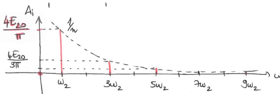
$$\text{Avec } \omega_2 = \frac{\omega_0}{3} = \frac{1}{3\sqrt{2}LC} = 2,36 \cdot 10^5 \text{ rad.s}^{-1}$$
