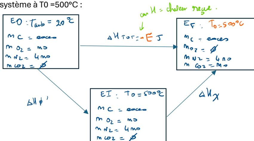
Alors  $-E = n_0(5 \times Cp(\text{Diatom})) \times (T_0 - T_{amb}) + n_0 \times \Delta rH^{\circ}$
