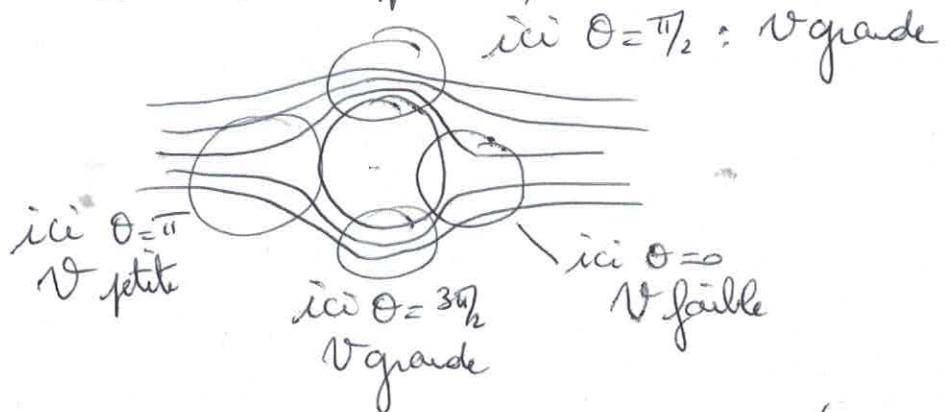
$$\vec{V}(r, \theta) = V_0 \left(1 - \frac{R^2}{r^2}\right) \cos \theta \hat{u} - \left(1 + \frac{R^2}{r^2}\right) V_0 \sin \theta \hat{e}_\theta$$
