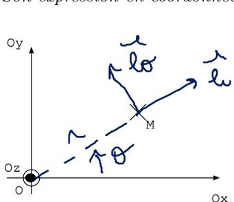
$$\begin{aligned} \vec{OM} &= r \vec{e}_r \\ \vec{v}(M)_{\mathcal{R}} &= \dot{r} \vec{e}_r + r \dot{\theta} \vec{e}_\theta \\ \vec{L}_O(M)_{\mathcal{R}} &= r \vec{e}_r \wedge m (\dot{r} \vec{e}_r + r \dot{\theta} \vec{e}_\theta) = m r^2 \dot{\theta} \vec{e}_z \end{aligned}$$
