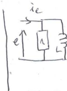
$$\begin{aligned} \underline{i}_e &= (\underline{Y}_n + \underline{Y}_L) \underline{e} \\ &= \left( \frac{1}{R_1} + \frac{1}{j\omega L} \right) \underline{e} \end{aligned}$$
