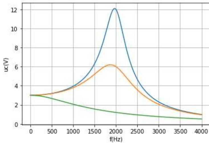
Réponses:  $E = 3 \text{ V}$ ,  $Q_3 = 4$  et  $f_0 = 2 \text{ kHz}$
