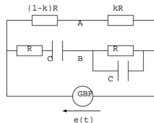
Réponses:  $\underline{Z}_1 \underline{Z}_3 = \underline{Z}_2 \underline{Z}_4$ ,  $k = 1/3$  et  $\omega = \frac{1}{RC}$
