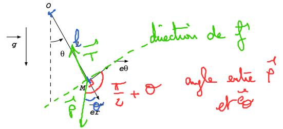
$$\begin{cases} \vec{OM} = l \vec{e}_r \\ \vec{v}(M) = l \frac{d\vec{e}_r}{dt} = l \dot{\theta} \vec{e}_\theta \\ \vec{a}(M) = l \left[ \ddot{\theta} \vec{e}_\theta + \dot{\theta} \frac{d\vec{e}_\theta}{dt} \right] = l \ddot{\theta} \vec{e}_\theta - l \dot{\theta}^2 \vec{e}_r \end{cases} \quad v = l \dot{\theta}$$
