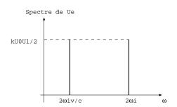
11. AN:  $\omega_i + \omega_r \approx 2\omega_i \approx 2,5.10^5 \ rad/s \ \text{et} \ |\omega_i - \omega_r| = \frac{2\omega_i V}{c} = 1500 \ rad/s.$
