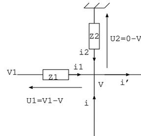
$$\text{On a } V = \frac{\frac{V_1}{Z_1} + \frac{0}{Z_2} + i - i'}{\frac{1}{Z_1} + \frac{1}{Z_2}}$$
