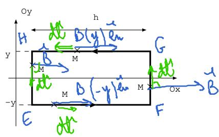
$$\begin{aligned} \oint \vec{B}(y) \cdot \hat{e}_n \, dl &= \int_E^F \vec{B}(y) \cdot \hat{e}_n \, dl + \int_G^H \vec{B}(y) \cdot \hat{e}_n \, dl + \int_H^E \vec{B}(-y) \cdot \hat{e}_n \, dl + \int_F^G \vec{B}(-y) \cdot \hat{e}_n \, dl \\ &= (B(-y) - B(y))h = -2B(y)h \quad \text{car } B(-y) = -B(y) \end{aligned}$$
