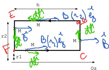
$$\begin{aligned} \oint \vec{B}(\mu) d\vec{l} &= \int_{\text{CD}} B(r_2) \hat{e}_z dl + \int_{\text{EF}} B(r_2) \hat{e}_y (-dl \hat{e}_y) + \int_{\text{FG}} B(r_1) \hat{e}_y dl \hat{e}_y \\ &= -B(r_2) h + B(r_1) h \end{aligned}$$
