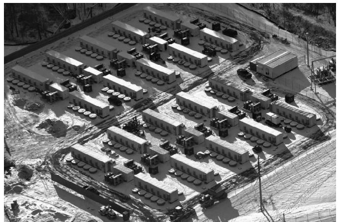
Figure 2 - Centrale inertielle de 20 MW, 2011, New-York, © Beacon Power.
