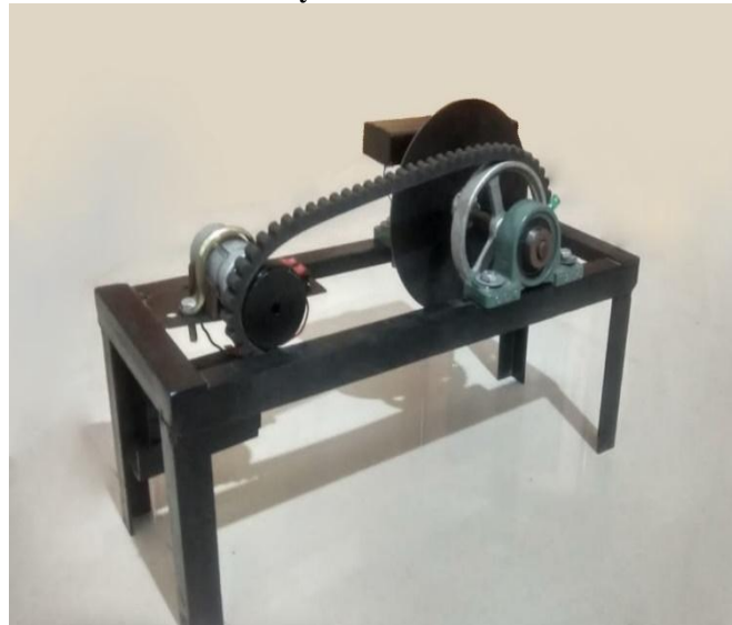
Fig 5.1 (Fabricated model of electromagnetic braking system)
