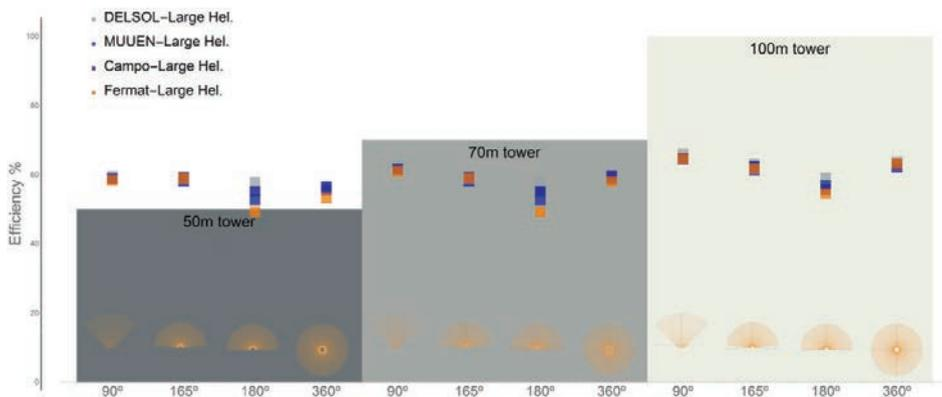
Figure 3: Annual efficiency of each algorithm for each scenario (90, 165, 180 and 360 Degree solar field acceptance angles and 50, 70, 100 m tower heights) for 140 m<sup>2</sup> heliostats.
