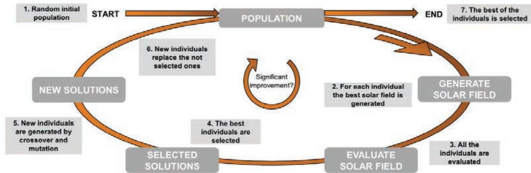
Fig. 1. Schematic representation of the solar field layout algorithms optimization procedure based on the “Backtracking Search Optimization Algorithm” (BSA) [16].
