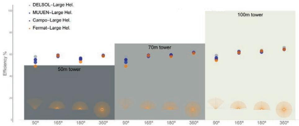
Figure 2: Annual efficiency of each algorithm for each scenario (90, 165, 180 and 360 Degree solar field acceptance angles and 50, 70, 100 m tower heights) for 140 m<sup>2</sup> heliostats.
