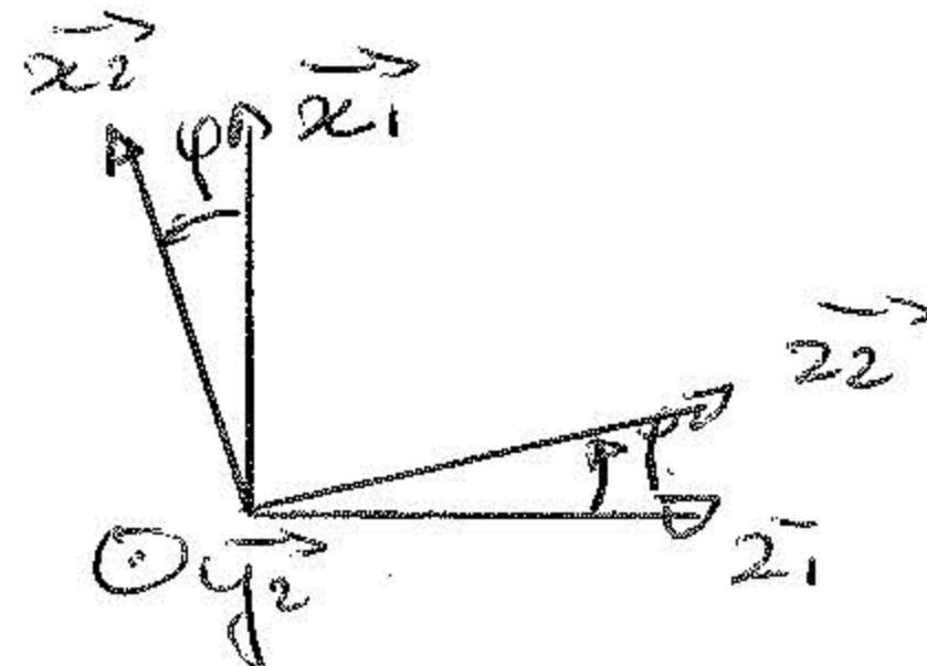
$$Q13) \quad \vec{z}_2 = \cos \varphi \vec{x}_1 + \sin \varphi \vec{x}_2.$$
