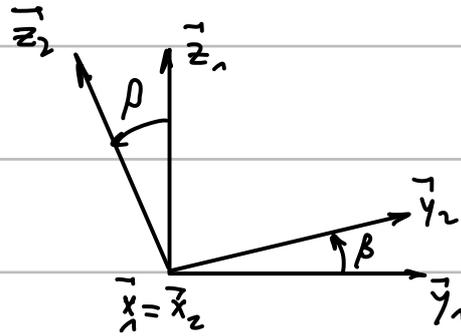
Q2 :  $\vec{\Omega}_{2/1} = \dot{\beta} \vec{x}_{12}$      $\vec{\Omega}_{1/0} = \dot{\theta} \vec{y}_{01}$      $\vec{\Omega}_{2/0} = \vec{\Omega}_{2/1} + \vec{\Omega}_{1/0}$
