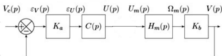
$$H_n(p) = \frac{V(p)}{V_c(p)} = \frac{k_a C(p) H_m(p) K_b}{1 + k_a C(p) H_m(p) K_b} = \frac{k_a k_b C H_m(p)}{1 + k_a k_b C H_m(p)}$$
