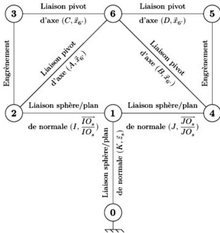
Q2: On cherche  $\left\{ \mathcal{V}_{0/1} \right\}_A = \left\{ \begin{matrix} \vec{x}_{6/1} \\ \vec{v}_{AE6/1} \end{matrix} \right\}_A = \left\{ \begin{matrix} p_{61} \vec{x}'_6 + r_{61} \vec{z}'_6 \\ \vec{0} + \vec{A}\omega_1 (p_{61} \vec{x}'_6 + r_{61} \vec{z}'_6) \end{matrix} \right\}_A$
