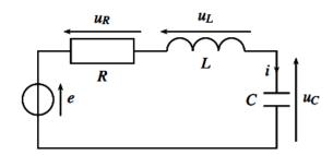
$$\underline{\mathbf{u}_{C}} = \frac{\underline{\mathbf{Z}_{C}}}{\underline{\mathbf{Z}_{R}} + \underline{\mathbf{Z}_{C}} + \underline{\mathbf{Z}_{L}}} \mathbf{e} = \frac{\frac{1}{jC\omega}}{R + \frac{1}{jC\omega} + jL\omega} \mathbf{e} = \frac{1}{-LC\omega^{2} + 1 + jRC\omega} \mathbf{e}$$
