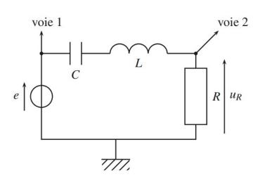
$$\underline{u}_{R} = \frac{\underline{Z}_{R}}{\underline{Z}_{R} + \underline{Z}_{L} + \underline{Z}_{c}} \underline{e} \Rightarrow \underline{u}_{R} = \frac{R}{R + jL \omega + \frac{1}{jC \omega}} \underline{e}$$
