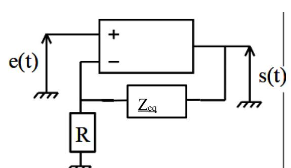
$$\underline{Z}_{eq} = \frac{1}{\frac{1}{Z_c} + \frac{1}{R}} = \frac{1}{jC\omega + \frac{1}{R}} \Rightarrow \underline{Z}_{eq} = \frac{R'}{1 + jR'C\omega}$$
