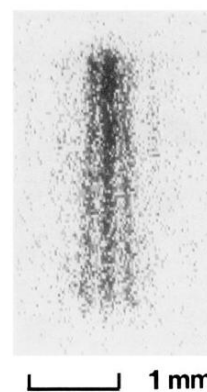
FIG. 2. The interference fringe pattern on the MCP for atoms with the initial velocity of approximately zero. The vertical length of the slit image is 2.8 mm. The spatial resolution of the picture is 20 and 32 \mu\text{m} for the horizontal and vertical directions, respectively. The narrowing of the fringe separation on the upper part is due to the damage of the double-slit structure. This figure contains approximately 6 \times 10^3 atomic counts.
