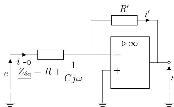
$$\begin{aligned} \frac{e - 0}{Z_{\text{éq}}} &= \frac{i' - 0 - s}{R'} \\ \frac{s}{e} &= -\frac{R'}{Z_{\text{éq}}} \\ \underline{H} &= -\frac{R'}{R + \frac{1}{Cj\omega}} \\ &= -\frac{\frac{R'}{R}}{1 - j \frac{1}{RC\omega}} \end{aligned}$$
