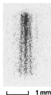
FIG. 2. The interference fringe pattern on the MCP for atoms with the initial velocity of approximately zero. The vertical length of the slit image is 2.8 \mu\text{m} . The spatial resolution of the picture is 20 and 32 \mu\text{m} for the horizontal and vertical directions, respectively. The narrowing of the fringe separation on the upper part is due to the damage of the double-slit structure. This figure contains approximately 6 \times 10^3 atomic counts.
