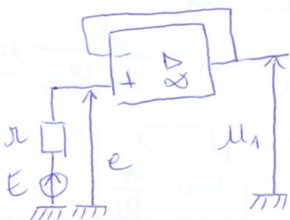
$$e = v_+ = v_- = u_1 \quad (\Rightarrow) \quad u_1 = e$$
