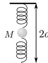
**Rép :**  $\ell_{1/2} = a \pm \frac{mg}{2k}$ , oscillations à  $\omega_0 = \sqrt{\frac{2k(1 - \ell_0/a)}{m}}$
