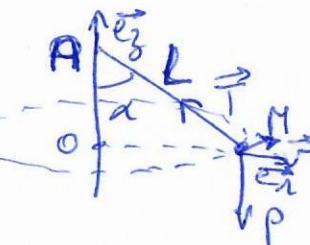
$$\begin{aligned} 2) \vec{J}_A(\vec{T}) &= \vec{AM} \times \vec{v} = (-l\omega \sin \theta \hat{e}_z + l\sin \theta \hat{e}_x) \times (l\cos \theta \omega \hat{e}_y) \\ &= l^2 m \omega \sin \theta (\cos \theta \hat{e}_x + \sin \theta \hat{e}_y) \end{aligned}$$
