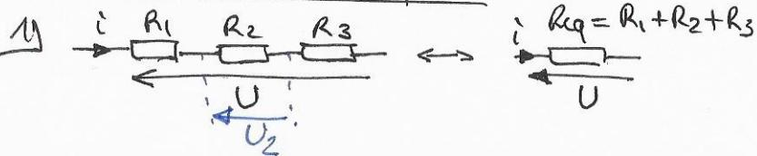
$$\text{Démon: } U = R_1 i + R_2 i + R_3 i = (R_1 + R_2 + R_3) i = \text{Req } i.$$
