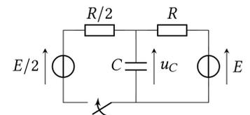
**Rép :**  $\frac{du_C}{dt} + 3\frac{u_C}{RC} = \frac{2E}{RC}; \tau = \frac{RC}{3}; u_C = \frac{E}{3}(e^{-t/\tau} + 2); t_1 = 3,9\tau; P_{tot} = \frac{E^2}{9R}(3e^{-2t/\tau} - 4e^{-t/\tau} + \frac{3}{2})$
