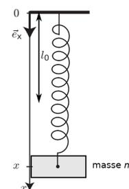
**Rép :**  $\ddot{x} + \frac{k}{m}(x - l_0) = g$ ;  $x_{\text{eq}} = l_0 + \frac{mg}{k}$ ;  $\ddot{u} + \omega_0^2 u = 0$ ,  $\omega_0 = \sqrt{\frac{k}{m}}$ ;  $u = \delta \cos \omega_0 t$ ;  $T = 2\pi \sqrt{\frac{m}{k}}$
