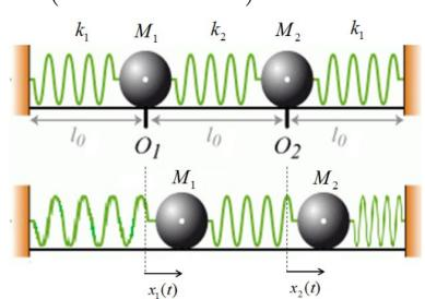
On pose  $\omega_S = \sqrt{\frac{k_1}{m}}$  et  $\omega_A = \sqrt{\frac{k_1 + 2k_2}{m}}$ .
