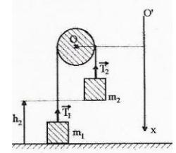
Rép : 1.  $\gamma_2 = \frac{m_2 - m_1}{m_2 + m_1} g; \gamma_1 = -\frac{m_2 - m_1}{m_2 + m_1} g$  2.  $t = \sqrt{\frac{2h_2}{\gamma_2}} = \sqrt{\frac{2h_2(m_1 + m_2)}{(m_2 - m_1)g}}$   $v_2 = \sqrt{\gamma_2 h_2}; v_1 = -\sqrt{2\gamma_2 h_2}$
