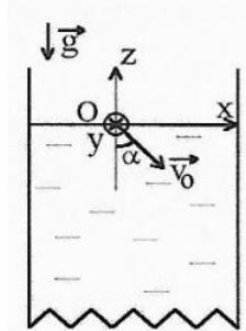
Rép :  $v_x = v_0 \sin \alpha e^{-\frac{9}{2} \frac{\eta}{r^2 \mu} t}$   $v_z = -\frac{2}{9} \frac{r^2}{\eta} (\mu - \mu_1) g \left(1 - e^{-\frac{9}{2} \frac{\eta}{r^2 \mu} t}\right) - v_0 \cos \alpha e^{-\frac{9}{2} \frac{\eta}{r^2 \mu} t}$ ;  $x = \frac{v_0 \sin \alpha}{\beta} \left(1 - e^{-\beta t}\right)$ ;  $z = -\frac{(\mu - \mu_1)g}{\beta \mu} \left(t + \frac{e^{-\beta t} - 1}{\beta}\right) + \frac{v_0 \cos \alpha}{\beta} (e^{-\beta t} - 1)$
