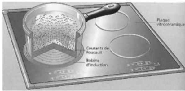
Figure 1 - Plaque à induction
