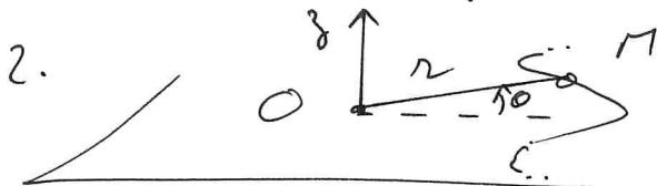
$$\begin{aligned} \vec{L} &= r \hat{e}_r \wedge (m r \hat{e}_r - m r \dot{\theta} \hat{e}_\theta) \\ &= m r^2 \dot{\theta} \hat{e}_z \quad (\text{car } z=0). \end{aligned}$$
