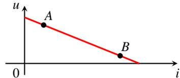
$$-r = \frac{\Delta u}{\Delta i} = \frac{u_B - u_A}{i_B - i_A} \iff r = -\frac{u_B - u_A}{i_B - i_A}$$
