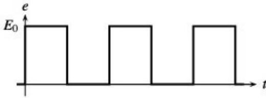
$$e(t) = \frac{E_0}{2} + \frac{2E_0}{\pi} \sum_{n=1,3,5,\dots} \frac{1}{n} \sin\left(n \times 2\pi \frac{t}{T_e}\right)$$
