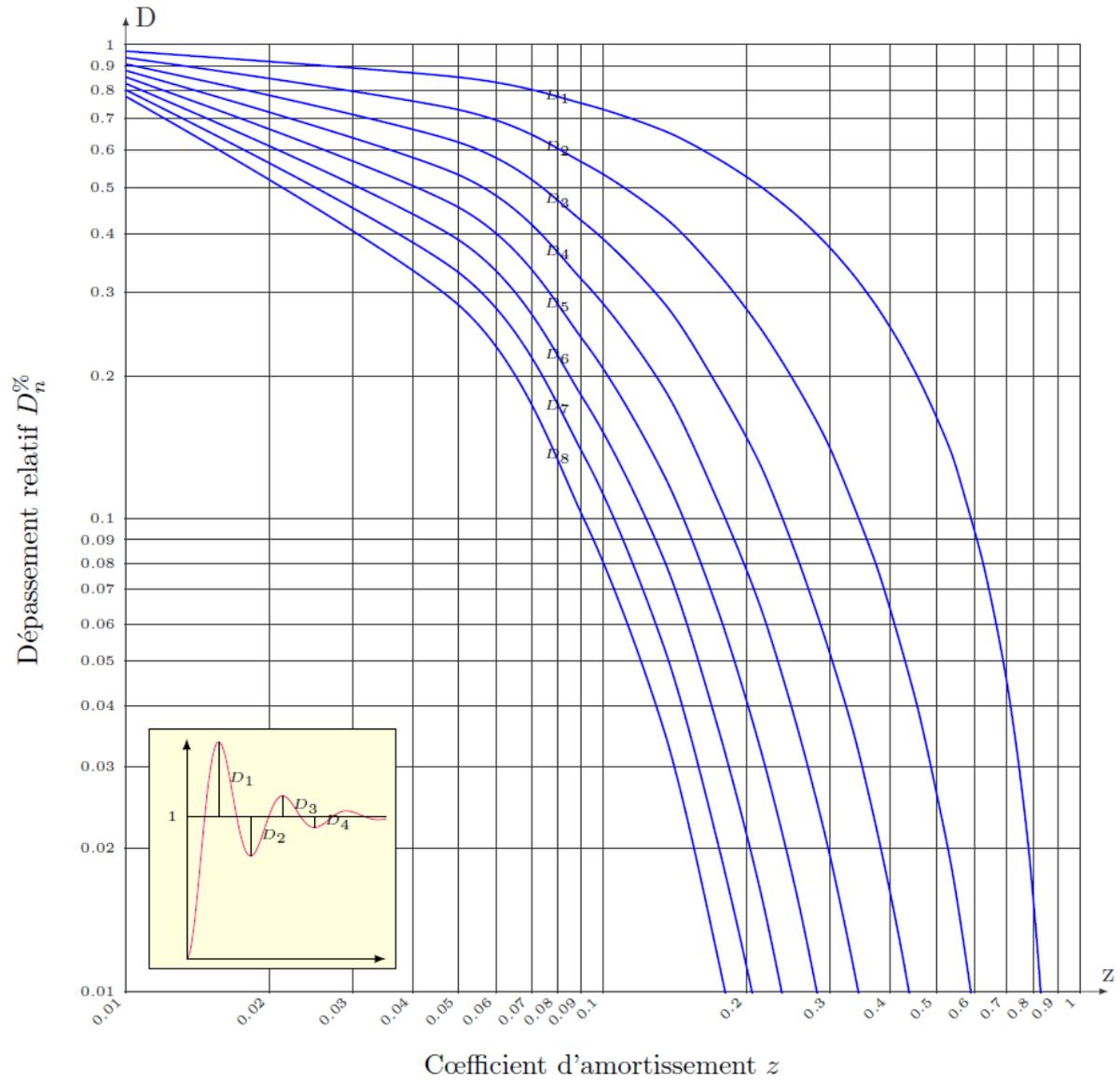
ABAQUE DU TEMPS DE REPONSE REDUIT  $t_{5\%} \cdot \omega_0$
