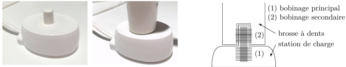
Figure 9 Station de charge
