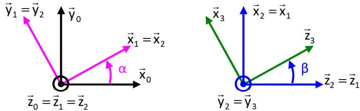
$$\mathbf{Q.3.} \quad \overrightarrow{V_{G,3/0}} = \overrightarrow{V_{G,3/0}} = \frac{d}{dt} \overrightarrow{OG} \Big|_0 = \frac{d}{dt} \left. \lambda(t) \cdot \vec{z}_0 + a \cdot \vec{x}_1 + b \cdot \vec{x}_1 + l \cdot \vec{x}_3 \right|_0 = \dot{\lambda}(t) \cdot \vec{z}_0 + (a+b) \cdot \dot{\alpha} \cdot \vec{y}_1 + l \cdot \frac{d}{dt} \vec{x}_3 \Big|_0$$
