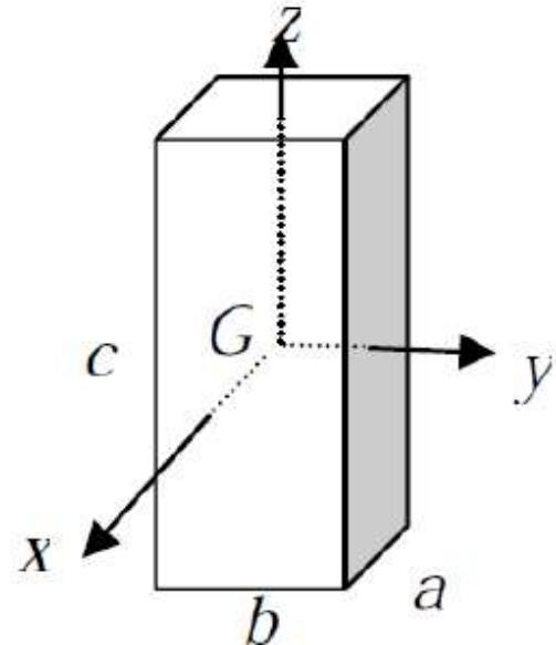
$$I(G, S) = \begin{bmatrix} \frac{m(b^2 + c^2)}{12} & 0 & 0 \\ 0 & \frac{m(a^2 + c^2)}{12} & 0 \\ 0 & 0 & \frac{m(b^2 + a^2)}{12} \end{bmatrix}_{(\bar{x}, \bar{y}, \bar{z})}$$
