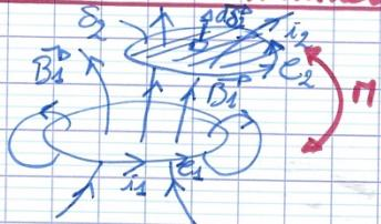
$$\Phi_{1 \rightarrow 2} = \iint_{S_2} B_1 \cdot dS_2 \quad \text{SD} \quad \Phi_{1 \rightarrow 2} = M i_1$$
