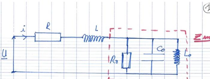
$$Q = R_0 C_0 \omega_0 = \frac{\sqrt{mk}}{\lambda}$$
