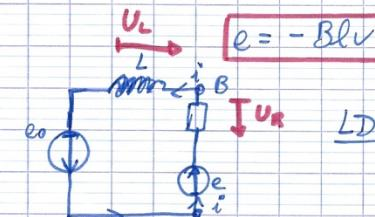
$$\text{LDM: } e + e_0 = U_R + U_L = R_i + L \frac{di}{dt}$$
