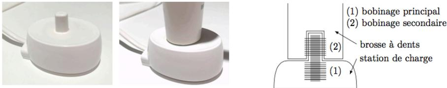
Figure 9 Station de charge
