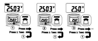
Note - The Range button is pressed to select manual ranging and to change ranges. When the Range button is pressed once, the AUTO indicator turns off. Press the Range button to select the appropriate range for the measurement you want to make. Press the Range button and hold for 1 second to return to Autorange mode.
