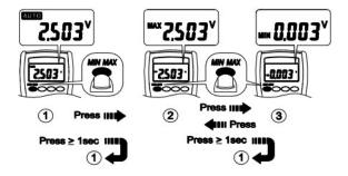
Note – Press the *HOLD* button in *MIN MAX* mode to make the meter stop updating the maximum and minimum value. When display *Hold* mode is nested in *MIN MAX* mode, the *MIN MAX* mode must be released before the display Hold.
