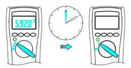
Note – If the meter idles for more than 10 minutes, the meter automatically turns the power off. When this happens, the LCD displaying-state of the meter is saved. The meter can be turned back on by pushing any button, the LCD displays the saved state. Pushing *Hold* button to disables the hold state. Any button press or rotary switch change resets the time of Auto Power-OFF.
