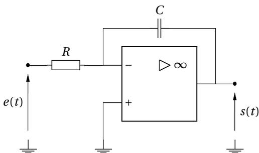
$$\underline{H}(j\omega) = -\frac{1}{j\omega\tau} \quad \text{avec} \quad \tau = RC,$$
