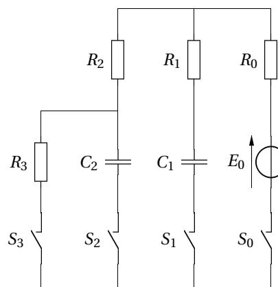
On donne  $R_0 = 50 \Omega$ ;  $R_1 = R_2 = R_3 = 25 \Omega$ ;  $E_0 = 10 \text{ V}$ ;  $C_1 = 1 \mu\text{F}$  et  $C_2 = 4 \mu\text{F}$ .
