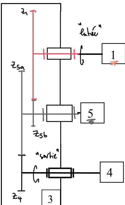
$$\begin{aligned} n &= \frac{\omega_{4/3}}{\omega_{1/3}} = \frac{\text{"sortie"}}{\text{"entrée"}} \\ &= \frac{z_1}{z_{5b}} \cdot \frac{z_{5a}}{z_4} \\ &= \frac{68}{17} \cdot \frac{57}{17} \approx \frac{3900}{290} \end{aligned}$$
