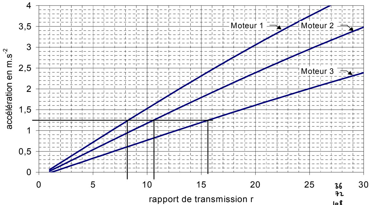
$$\text{On veut: } a = \frac{45 - 0}{10} \frac{(\text{km/h})}{(\text{s})} = \frac{4,5}{3,6} = 1,25 \text{ m/s}^2$$
