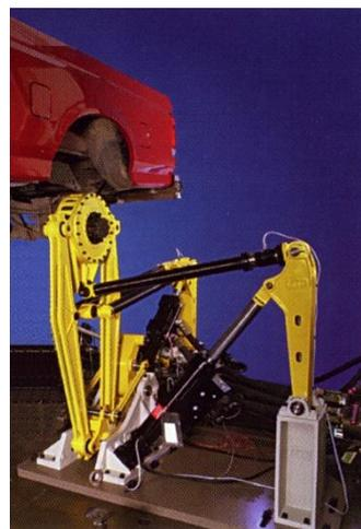
Figure N°3 : Ensemble roue-suspension + MTS Model 329
