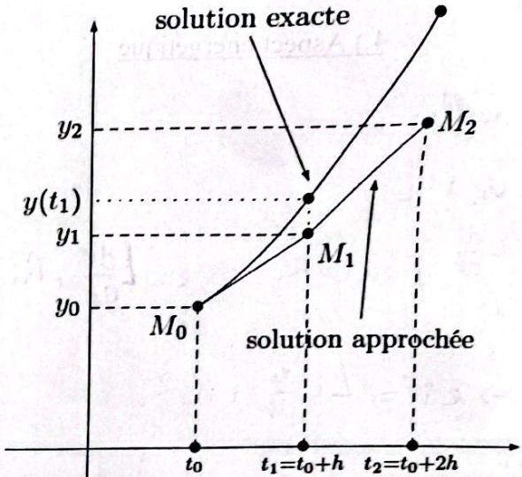
$$\begin{aligned} \text{eq. Tang. courbe.} \quad & \star \star \star \\ \left( \frac{du_c}{dt} \right) (t_h) &= \frac{U_{C,t_{h+1}} - U_{C,t_h}}{t_{h+1} - t_h} \\ \Rightarrow U_{C,t_{h+1}} &= \left( \frac{du_c}{dt} \right) (t_h) \times (t_{h+1} - t_h) + U_{C,t_h} \quad t_h = t_{h+1} - t_h \\ \Rightarrow U_{C,t_{h+1}} &= \frac{E - U_{C,t_h}}{C} \times h + U_{C,t_h} \quad \text{et } \frac{du_c}{dt} = \frac{E - U_C}{C} \end{aligned}$$
