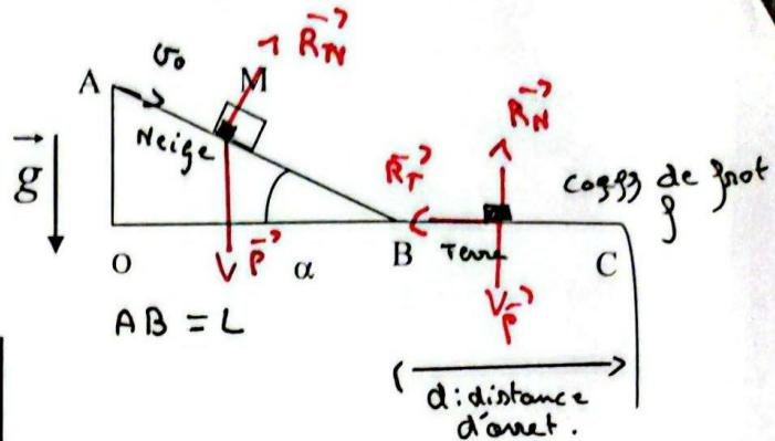
$$\Delta E_m = mg(z_C - z_A) - \frac{1}{2} m v_0^2$$
