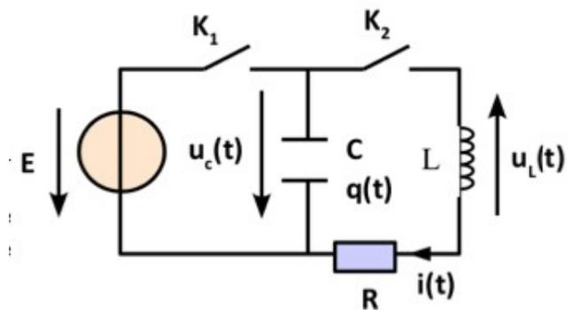
$$L = 10 \text{ mH} ; C = 0.1 \text{ } \mu\text{F} ; R \text{ variable.}$$
