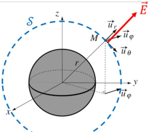
$$\int_0^{2\pi} d\varphi \int_0^\pi E(r) \vec{u}_r \cdot \vec{u}_r r^2 \sin \theta d\theta d\varphi = \frac{Q}{\varepsilon_0}$$
