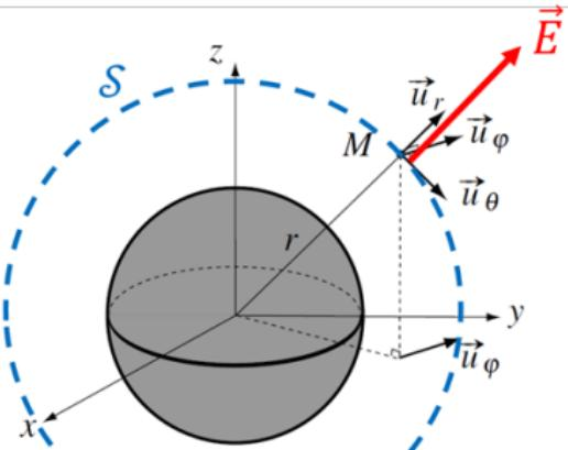
$$\int_0^{2\pi} d\varphi \int_0^\pi E(r) \vec{u}_r \cdot \vec{u}_r r^2 \sin \theta d\theta d\varphi = \frac{Q}{\varepsilon_0}$$
